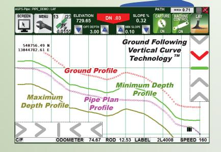
AGPS-Pipe Pro loads any geo-referenced data and maps to be used for guidance and planning.
